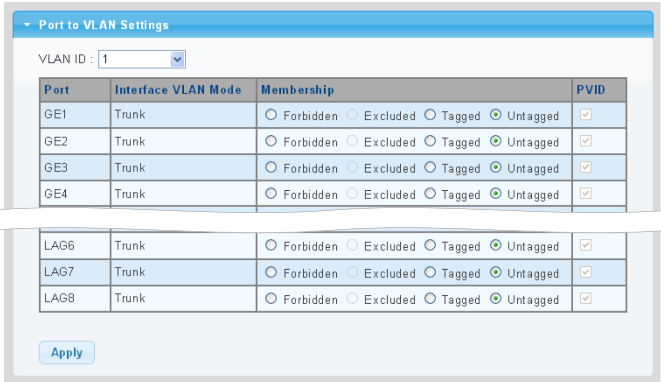
Figure 4-5-7: Port to VLAN Setting Page Screenshot
